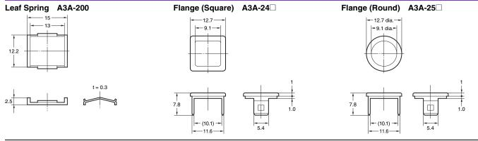
Note: Unless otherwise specified, a tolerance of  $\pm 0.4$  mm applies to all dimensions.
