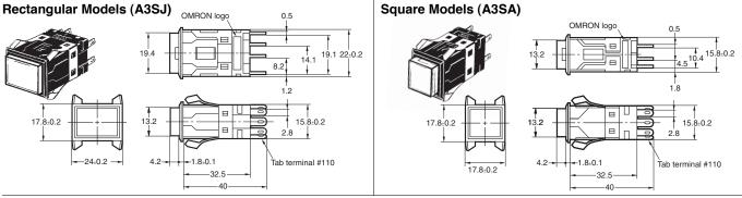
Note: Unless specified, a tolerance of ±0.4 mm applies for all dimensions. Use a mounting panel thickness of 1 to 4 mm.
