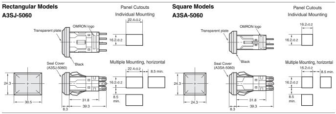
Note: 1. Recommended panel thickness: 1.0 to 3.3 mm
