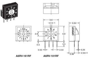
■ Top-actuated Extended-actuator Models with 4×1 Terminal Arrangement
