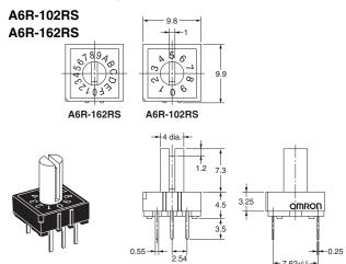
● Side-actuated Extended-actuator Models with 4×1 Terminal Arrangement
