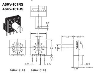
Note: Unless otherwise specified, a tolerance of ±0.4 mm applies to all dimensions.
