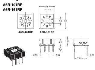
● Top-actuated Flat Models with 3×3 Terminal Arrangement
