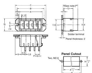
Note: If the output code is 06, the dimension is 19; if the output code is 07, the dimension is 31.
