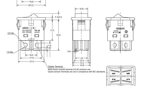
Note: Unless otherwise specified, a tolerance of ±0.3 mm applies to all dimensions.
