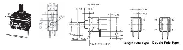
Note: Unless otherwise specified, a tolerance of ±0.4 mm applies to all dimensions.
