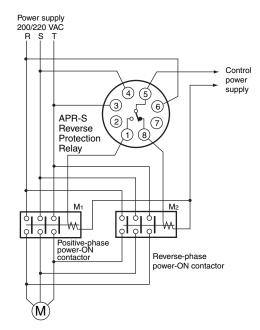
Suppose the motor revolves in the forward direction when the input terminals 6, 4, and 3 of the APR-S are connected, in this sequence to the power lines, R, S, and T, respectively. If the phase sequence of the power supply applied is the positive sequence, the relay built into the APR-S will turn ON, there will be continuity between terminals 5 and 1, and the positive-phase power-ON contactor will be energized.
