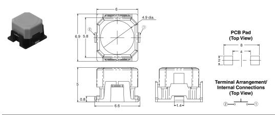
$\textbf{Note:} \quad \text{Unless otherwise specified, a tolerance of $\pm 0.4$ mm applies to all dimensions. No terminal numbers are indicated on the Switches.}$
