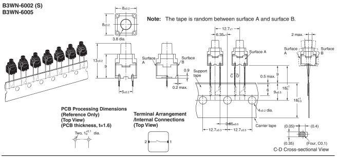
Note: Unless otherwise specified, a tolerance of ±0.4 mm applies to all dimensions. No terminal numbers are indicated on the Switches.
