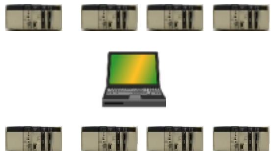
ControllerLink Module allows large amounts of high speed data to be exchanged between multiple Omron PLCs or a personal computer via the ControllerLink Network
