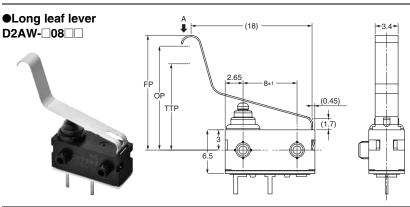
Operating Without Models with Туре characteristics Posts posts OF Max. 0.90N {91 gf} **Operating Force** Releasing Force RF Min. 0.05N {5 gf} Overtravel OT 2.8 mm (reference value) Movement Differential MD Max. 0.7 mm Free Position FP 19.0 mm Max. 23.0 mm **Operating Position** OP 19.4 ± 1.5 mm  $15.4\pm1.5$  mm Total Travel Position TTP 16.8 mm 12.8 mm
