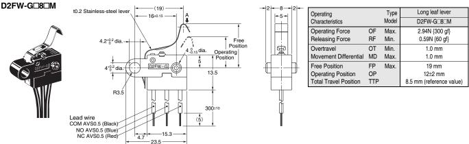
Note1. Unless otherwise specified, a tolerance of ±0.4 mm applies to all dimensions. Note2. The operating characteristics are for operation in the A direction ( -).
