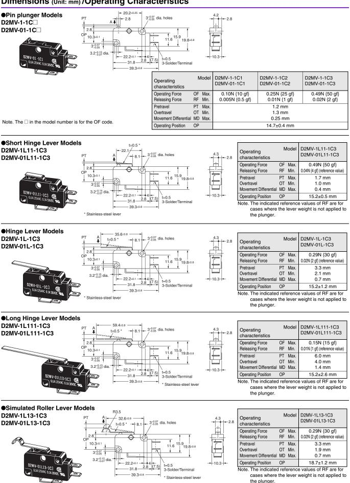
Note 1. Unless otherwise specified, a tolerance of ±0.4 mm applies to all dimensions. Note 2. The operating characteristics are for operation in the A direction ( 1).
