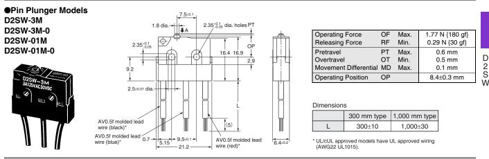
Note 1. Unless otherwise specified, a tolerance of  $\pm 0.4$  mm applies to all dimensions. Note 2. The operating characteristics are for operation in the A direction ( $\clubsuit$ ).
