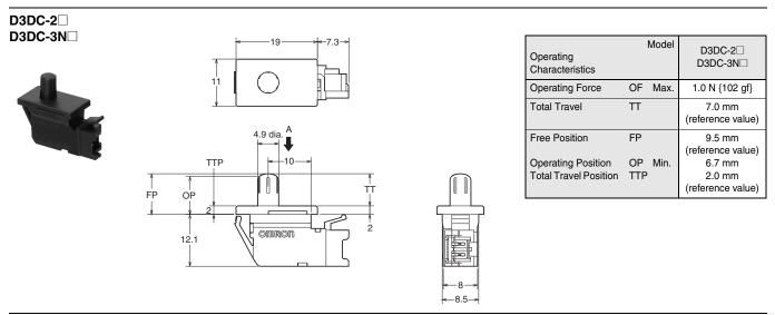
Note 1. Unless otherwise specified, a tolerance of  $\pm 0.4$  mm applies to all dimensions. Note 2. The operating characteristics are for operation in direction A ( $\clubsuit$ ).
