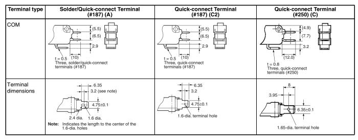
**Note:** The table above is for the SPDT contact specifications. Two terminals will be available for SPST-NO or SPST-NC contact specifications. For terminal positions, refer to the above *Contact Form*.
