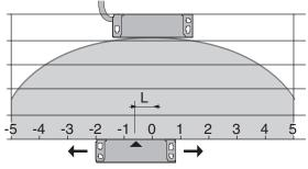
5 mm misalignment tolerance after setting
