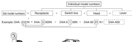
\* The D4A-□N without the above accessories is not compatible with the D4A-□.
