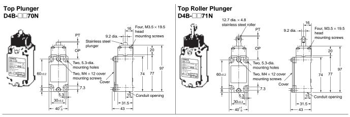
Note: Unless otherwise specified, a tolerance of  $\pm 0.4$  mm applies to all dimensions.
