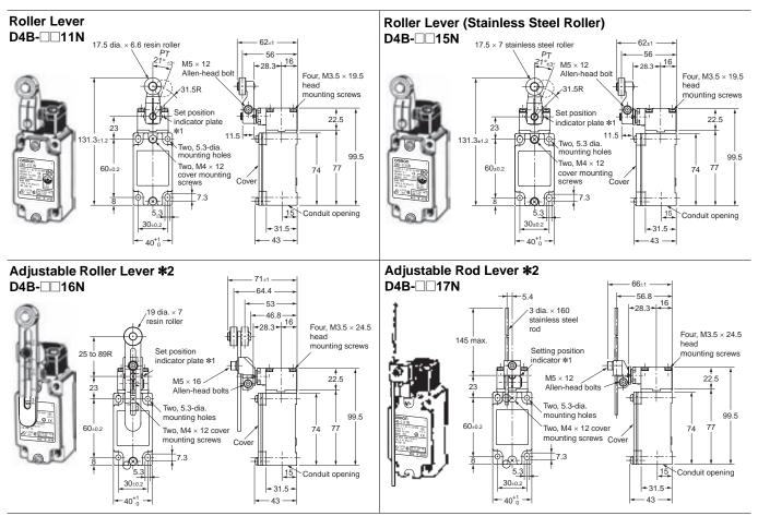
**Note:** Unless otherwise specified, a tolerance of  $\pm 0.4$  mm applies to all dimensions. **\*1.** The lever can be set to any desired position by turning the operating position indicator.
