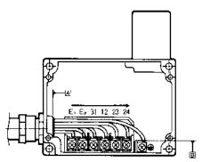
Tighten each wired terminal clockwise to a torque of 0.59 to 0.78 N·m.
