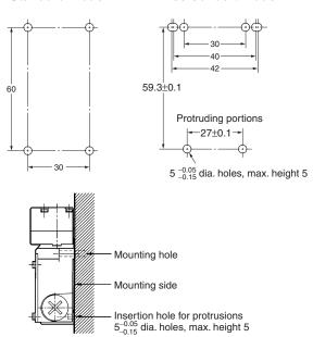
The D4BS can be mounted more securely by adding two protruding portions, each of which is 5 mm maximum in height and 5  $^{-0.05}/_{-0.15}$  mm in diameter as shown below.
