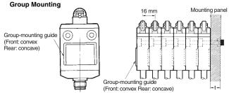
If the mounting panel is warped or has protruding parts, a malfunction may result. Make sure that the mounting panel is not warped and has even surfaces.
