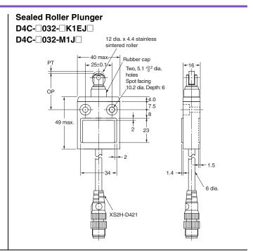
Note: Unless otherwise specified, a tolerance of  $\pm 0.4 \ \text{mm}$  applies to all dimensions.
