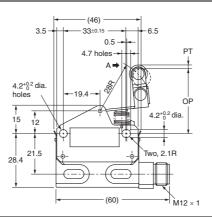
$9.5~\text{dia.} \times 4.0~\text{stainless}$ sintered alloy roller
