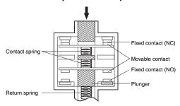
Conforms to EN60947-5-1 Direct Opening Operation ⊖
