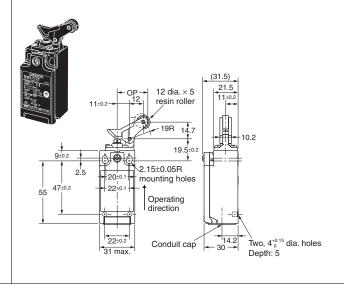
**Note:** Unless otherwise specified, a tolerance of  $\pm 0.4$  mm applies to all dimensions. \* Refer to page 12 for details on M12 connectors.
