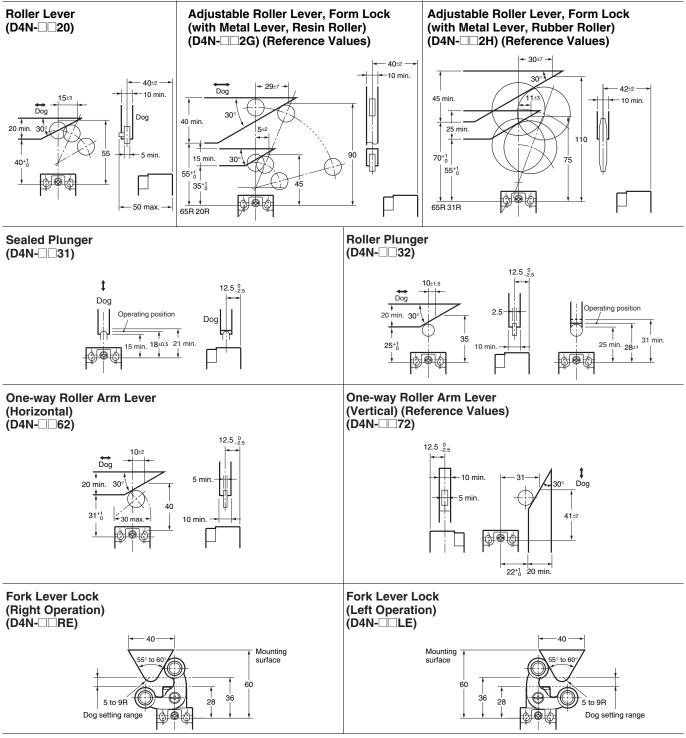
Note: Unless otherwise specified, a tolerance of  $\pm 0.4 \ \text{mm}$  applies to all dimensions.
