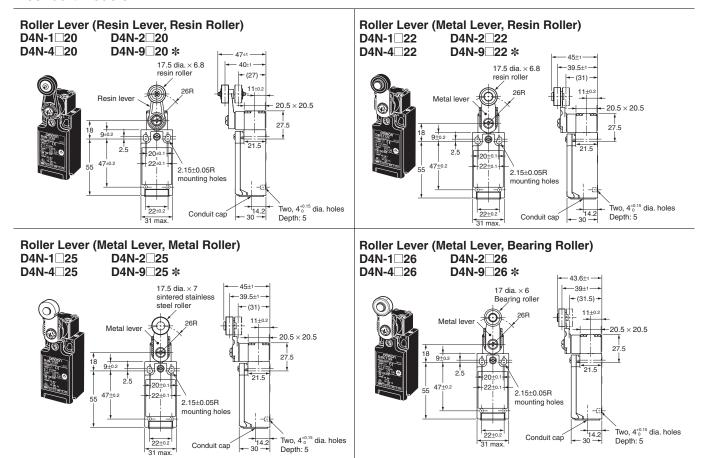
**Note:** Unless otherwise specified, a tolerance of  $\pm 0.4$  mm applies to all dimensions. \* Refer to page 12 for details on M12 connectors.
