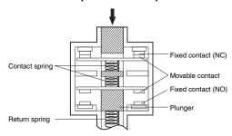
Conforms to EN60947-5-1 Direct Opening Operation ⊖
