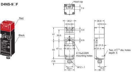
Operating characteristics Model D4NS-9□F Key insertion force 15 N max. Key extraction force 30 N max. Pretravel (PT) 6±3 mm Total travel (TT) (28 mm) Direct opening force \* Direct opening stroke \* 60 N min. 10 mm min
