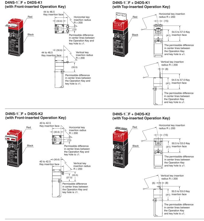
Note: Unless otherwise specified, a tolerance of ±0.4 mm applies to all dimensions.
