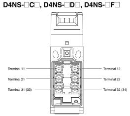
Note: The 2-conduit models have the same terminal arrangement.
