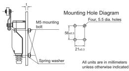
Note: The tap screws for the body are M5, P=0.8, with a minimum depth of 7.5 mm. Use bolts with a length of the panel thickness t + 7 mm or less.
