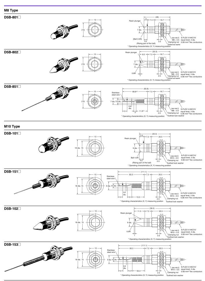
Note: 1. Unless otherwise specified, a tolerance of  $\pm 0.4$  mm applies to all dimensions.
