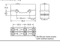
Dimensions and Operating Characteristics The solder terminal model has a suffix "-1A" in its model number and its omitted dimensions are the same as the corresponding dimensions of the pin plunger model.
