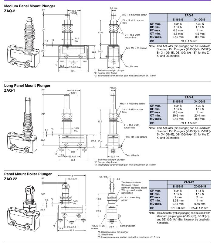
Note: Each dimension has a tolerance of ±0.4 mm unless otherwise specified.
