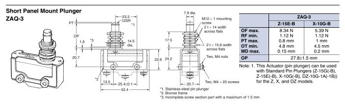
Note: Each dimension has a tolerance of  $\pm 0.4$  mm unless otherwise specified.
