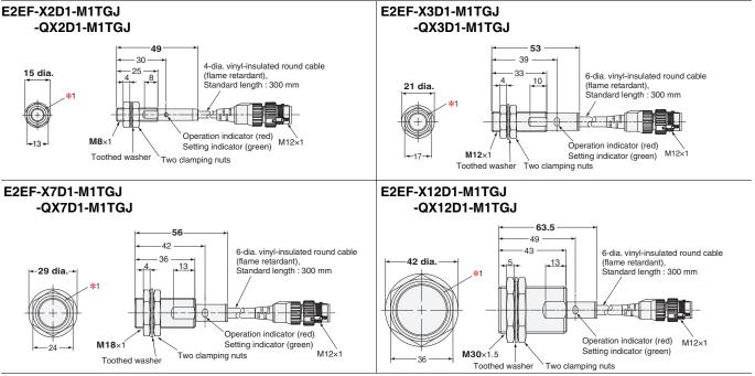
\*1. The E2EF-QX D type Clamping nut (optional accessory) is grooved to identify the material (SUS303, with fluororesin coating).
