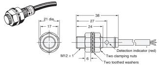
6-dia. vinyl-insulated round cable with 3 conductors (Flame resistant, Conductor cross section: 0.5 mm², Insulator diameter: 1.9 mm), Standard length: 2 m
