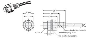
6-dia. vinyl-insulated round cable with 2 conductors (Flame resistant, Conductor cross section: 0.5 mm², Insulator diameter: 1.9 mm), Standard length: 2 m
