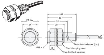
\* 6-dia. vinyl-insulated round cable with 3 conductors (Flame resistant, Conductor cross section: 0.5 mm2, Insulator diameter: 1.9 mm), Standard length: 2 m The cable can be extended up to 200 m (separate metal conduit).
