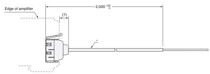
$^{\star} \ E3X-CN12; \textbf{2.6 dia.} \ cable \ / \ \textbf{1 conductor} \ / \ Standard \ length: 2 \ m \ (Conductor \ cross \ section: 0.2 \ mm^2 \ (AWG24), \ Insulator \ diameter: 1.1 \ mm)$
