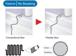
A large number of ultrafine cores are all surrounded by cladding. As a result, the fiber is flexible and can be bent without significantly reducing the light intensity. This helps solve problems, such as fiber being broken by getting caught on other objects.
