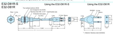
Note: The maximum allowable temperatures for sections A and B are 200°C and 110°C, respectively. The section inserted into the Amplifier Unit (indicated by \*2), however, must stay within the Amplifier Unit's operating temperature range.
