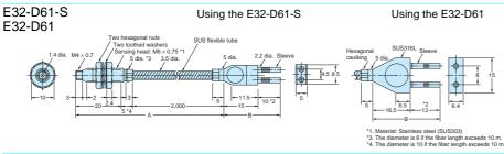
Note: The maximum allowable temperatures for sections A and B are 350°C and 110°C, respectively. The section inserted into the Amplifier Unit (indicated by \*2), however, must stay within the Amplifier Unit's operating temperature range.
