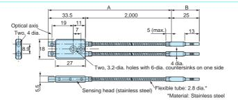
Note: The maximum allowable temperatures for sections A and B are 200°C and 110°C, respectively. The section inserted into the Amplifier Unit (indicated by \*2), however, must stay within the Amplifier Unit's operating temperature range.
