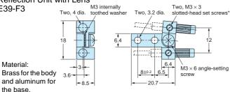
\*Secure the fiber head with the slotted-head set screws. Do not insert a lens (E39-F1).
