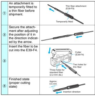
Note: Insert the fiber in the direction indicated by the arrow.
