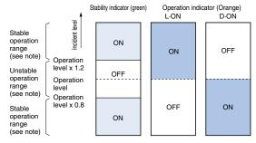
Note: If the operation level is set to the stable operation range, the E3G will operate with the highest reliability and without being influenced by temperature change, voltage fluctuation, dust, or setting change.
