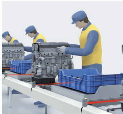
Presence detection of pallets
