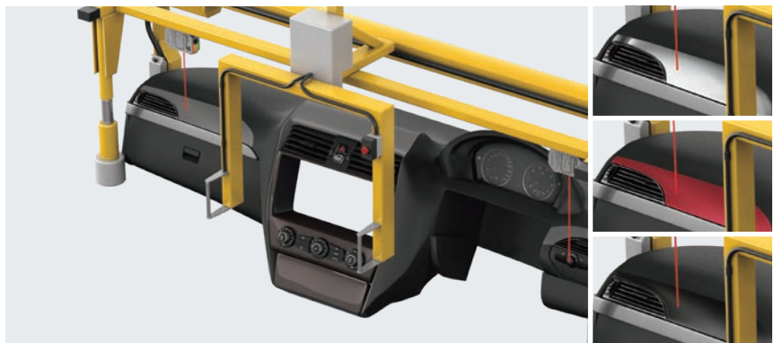
Presence detection of interior decoration parts
