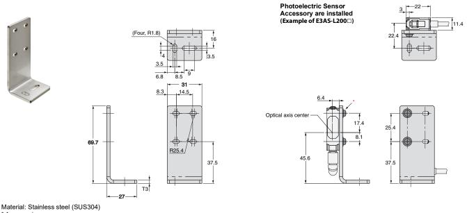
\* Accessories 2-M3-L12 Cross Recessed Pan Head Screws (Attached to SW+JIS W)
