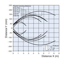
Retro-reflective Models (radial) E3F2-R2R□41-□ (polarizing) and reflectors
