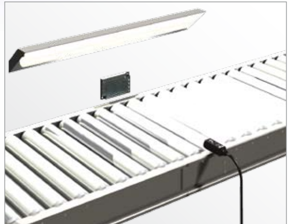
Pulse synchronisation for high ambient light immunity.
