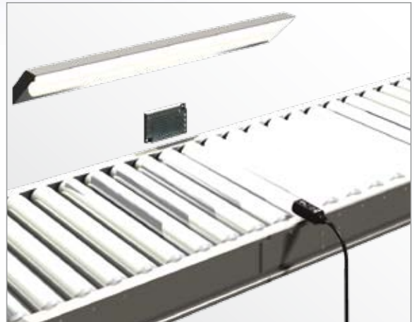
Pulse synchronisation for high ambient light immunity.
