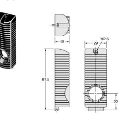
Terminal Protection Cover for Side-pullout Cable (Example of E3G-MR19-G)
