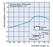
Sensing Object Angle (Left and Right)
