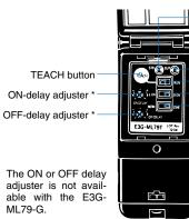
(Red and green) Operation indicator (Orange) TEACH/RUN selector L-ON/D-ON selector NORMAL/ZONE selector
