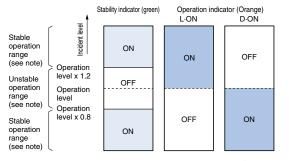
Note: If the operation level is set to the stable operation range, the E3G will operate with the highest reliability and without being influenced by temperature change, voltage fluctuation, dust, or setting change. Maximum distance setting (in normal mode) If you want to set the maximum distance of the sensor, set a maximum distance as depicted in the following procedure.
