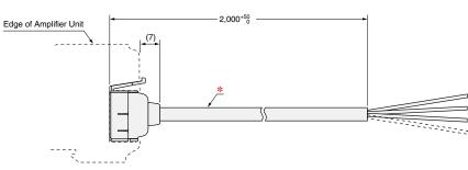
\* 4-dia. cable with 3 conductors, Standard cable length: 2 m (Conductor cross-section: 0.2 mm² (AWG24), Insulator diameter: 1.1 mm)
