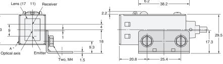
\*The Mounting Bracket can be attached to side A.
