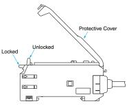
Note:To maintain the fiber properties, confirm that the lock is released before removing the fiber.
