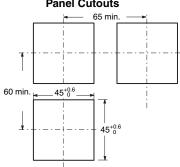
mounting space between each Unit. Units must not be closely mounted vertically or horizontally.
