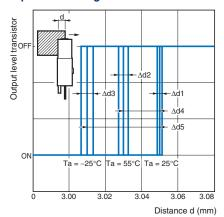
Vcc =12 V, No. of repetitions: 20,  $\Delta$ d1 = 0.002 mm,  $\Delta$ d2 = 0.004 mm,  $\Delta$ d3 = 0.005 mm,  $\Delta$ d4 = 0.02 mm,  $\Delta$ d5 = 0.04 mm
