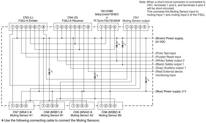
M12, 4-pin connector (Pin 1: +24 V, Pin 2: Not used, Pin 3: 0 V, Pin 4: Output) When using a Through-beam Photoelectric Sensor, use an XS2R-D426-[11-F Y-joint with Socket and Plug or similar product to connect the transmitter and receiver.
