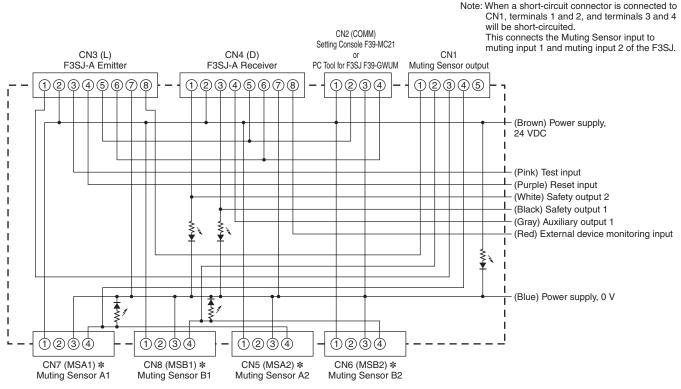
\* Use the following connecting cable to connect the Muting Sensors: M12, 4-pin connector (Pin 1: +24 V, Pin 2: Not used, Pin 3: 0 V, Pin 4: Output) When using a Through-beam Photoelectric Sensor, use an XS2R-D426-□11-F Y-joint with Socket and Plug or similar product to connect the transmitter and receiver.
