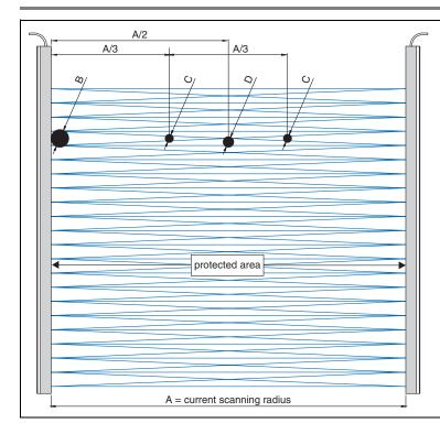
High resolution is realized by *triple crossing of light* beams.
