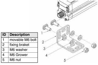
Note: Shipment contains different quantity of brackets, depending on the length of the SLC. Longer SLC contains a higher number of brackets, following the rule of every 400 mm one bracket.
