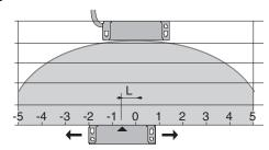
5 mm misalignment tolerance after setting
